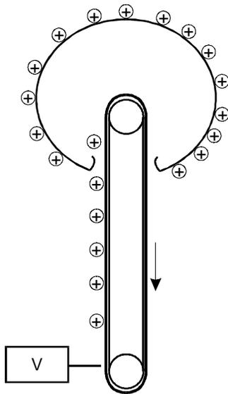
The diagram shows a Van de Graaff generator, which is a laboratory device for building up high voltage. The hollow metal sphere collects the charge while a belt carries charge from the voltage source to the sphere. The generator is 100% efficient and the potential difference between the belt and the sphere is 75 kV. Which of the following is the power needed to supply charge to the sphere at a rate of  $160 \mu\text{C/s}$ ?
