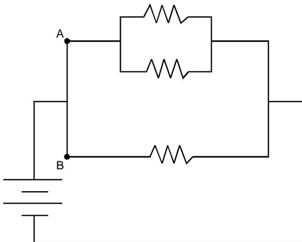
The diagram shows a circuit with three identical resistors. Which of the following is the ratio of the current through point *A* to the current through point *B*?
