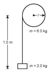
The diagram shows a frictionless wheel with a cable wrapped around it and a block attached to the end of the cable. The wheel has a mass of 6.0 kg and the block has a mass of 2.0 kg. The block is released from rest and drops as the cable unwinds. When the block has dropped 1.0 m, its velocity is 2.8 m/s. What is the kinetic energy of the wheel?
