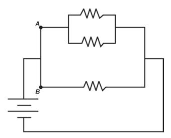
The diagram shows a circuit with three identical resistors. What is the ratio of the current through point A to the current through point B?
