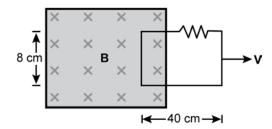
A loop of wire that measures 8 cm by 40 cm is attached to a 4  $\Omega$  resistor and is inside a uniform 0.5 T magnetic field that points into the computer screen. The loop is pulled out of the field at a constant speed of 5 cm/s. What is the magnitude and direction of the induced current in the loop?
