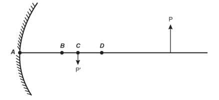
A curved mirror forms an image P' of an object P. Which of the following best indicates the location of the focal point of the mirror?
