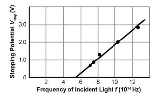
The graph shows data points and a fitted line in a photoelectric effect experiment. What is the work function for the metal in this experiment?
