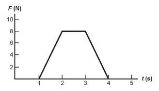
The graph shows the magnitude of a force as a function of time. At t = 0 s, a 10 kg object is moving at 4.0 m/s. The force shown on the graph is applied to the object in the direction of motion. What is the momentum of the object at t = 5 s?
