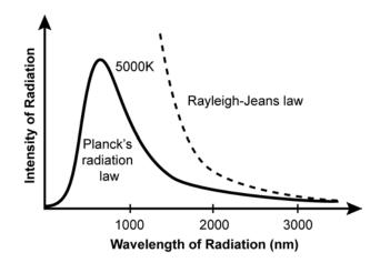
The diagram shows two models for how the intensity of the radiation by a blackbody depends on the wavelength of light. The Rayleigh-Jeans law predicted that the energy would become infinite as  $\lambda \rightarrow 0$ . Planck's radiation law better matched empirical evidence and showed the energy radiated goes to 0 as  $\lambda \rightarrow 0$ . Which of the following best describes Planck's hypothesis?
