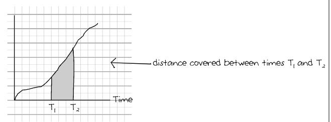
So, the area represents the total distance traveled between the two times. Slope = rise/run =  $\Delta v/\Delta t$  the rate of change of speed. This is acceleration, as shown in diagram below.
