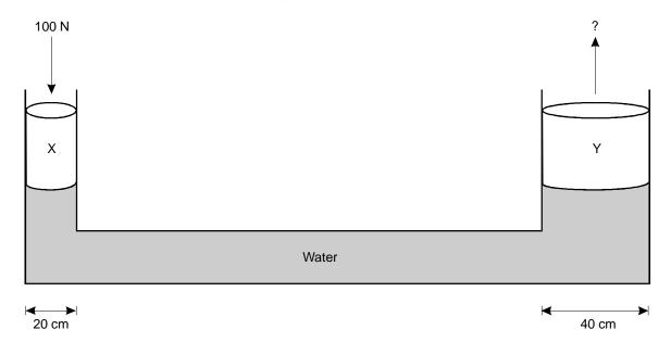
A force of 100 N is applied to piston X. What is the upward force applied by piston Y?
