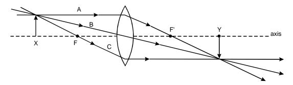
Ray A goes parallel to the axis from the arrow point to the lens and then is refracted through focal point F'. Ray B passes in a straight line directly through the center of the lens. Ray C passes from the arrow point through focal point F and then is refracted so it exits the lens parallel to the axis. The place where these rays converge indicates where the point of the projected arrow image will appear.
