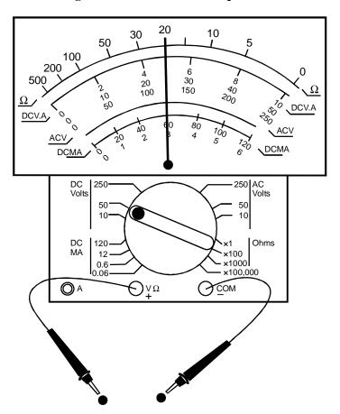
The multimeter in the diagram above is indicating a voltage of:
