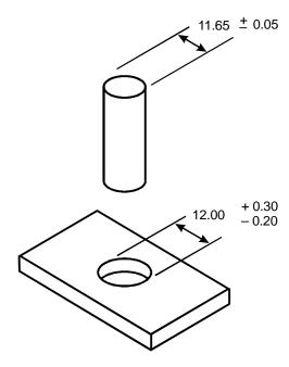
A machinist is to manufacture two parts as specified by the diagram above. According to the given tolerances, which of the following best describes the range of clearances between the two parts?
