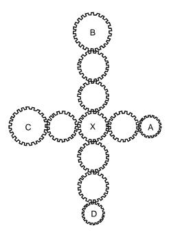
Which of the following gears in the diagram is rotating at a slower speed than, but in the same direction as, the gear labeled *X*?
