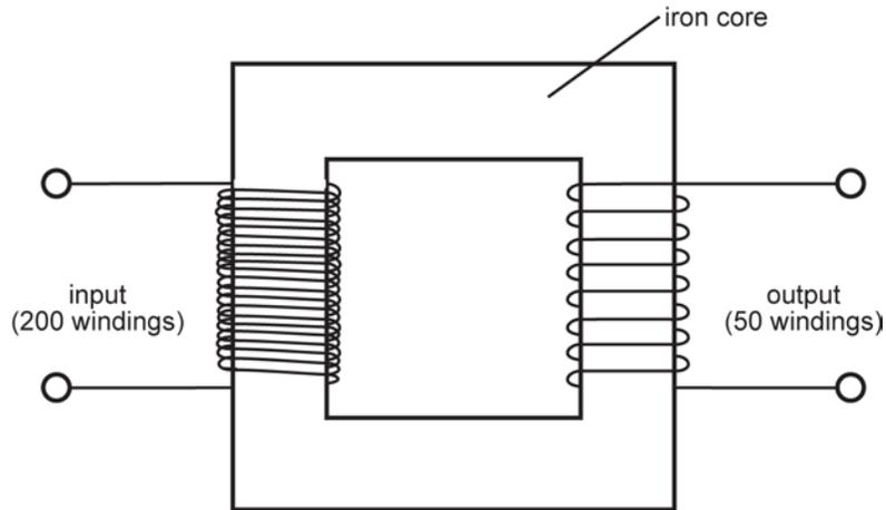
The device in the diagram consists of two windings of wire wrapped around an iron core. The windings are separate from each other, and neither is in direct contact with the other. There are 200 windings of wire on the input side and 50 windings of wire on the output side. The device most likely performs which of the following functions?
