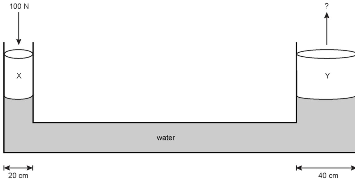
A force of 100 N is applied to piston X as shown in the diagram. What is the upward force applied by piston Y?
