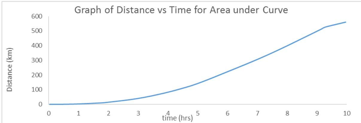
The total area under the curve of velocity vs time becomes the total distance covered by the train.
